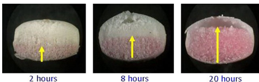
Fig. 3. Cross-section of felodipine PPOT using dibutyl sebacate as plasticizer after dissolution in time sequence
